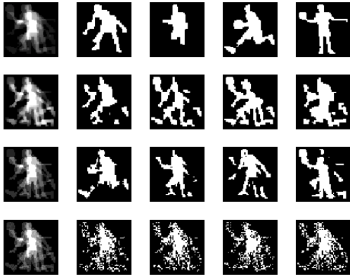
Figure 3: The average segmentation and samples from four models, one per line: perturbation model where the perturbations have unrestricted vs. diagonal covariance matrix and multivariate gaussian model with unrestricted vs. diagonal covariance matrix.
