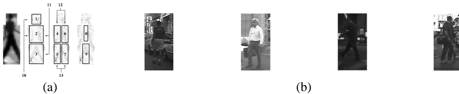
Figure 1: (a) The configuration of the nine sub-regions is displayed over the gradient image. (b) some of the positive examples — note the large variation in appearance, pose and articulation.
